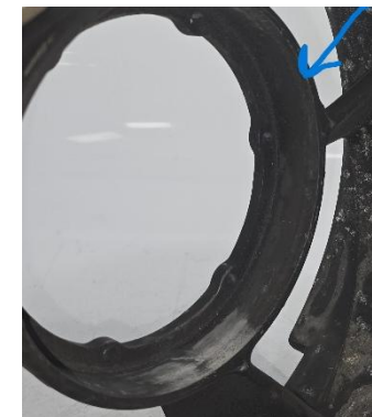
LMA064 / LMA333-2 Late 'thin' fan housing - 27mm lip
