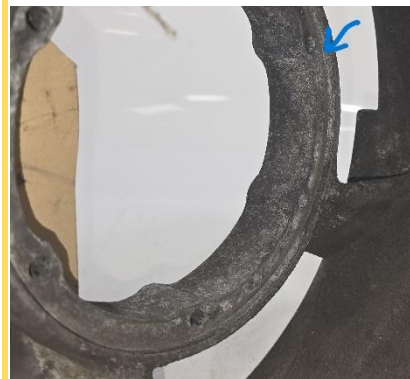
LMA036 / LMA333 early 'thick' fan housing - 7mm lip
