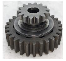
Above is a picture of the new WOSP starter ring gear fitted to the original Suzuki starter clutch.
