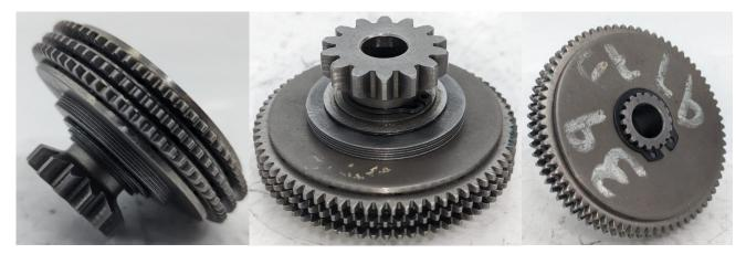
Above is pictures of the original starter clutch. There should be 5 x compression washers on the original part.
