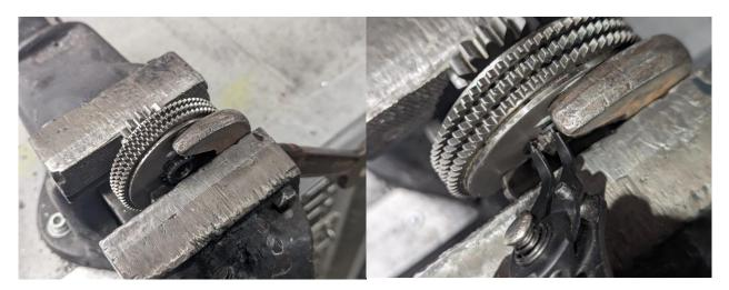
Remove the circlip from the original starter clutch. We used a spanner in the vice for compression.
