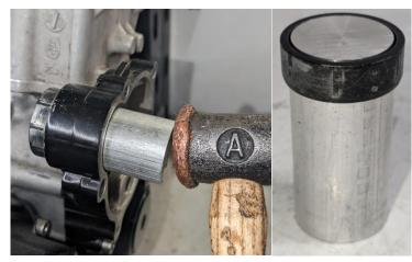
Using the tool we supplied remove the bush from the housing.
