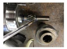
Slide the new drive back on to the splines and all the way back until it falls off the back of the spline and then move around and slide back up a locked section of splines meaning the drive can't come off.
