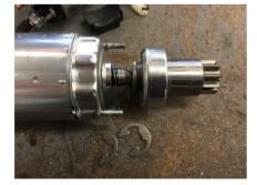
Knocking the c-clips off enables the drive to move back far enough to slide off the locked spline and on to the next spline which is open therefore enabling the drive to be taken off the shaft. Every other spline on the shaft is open, and every other spline is locked. For operation the drive needs to be on the locked splines so it cannot come off.
