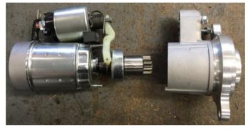
Push on the front of the pinion in order to remove the solenoid and motor assembly as one complete unit. It will make re-assembly easier and quicker if the unit stays complete.
