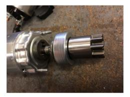
At this point re-fit the c-clips locking the drive on the locked spline section of the shaft.
