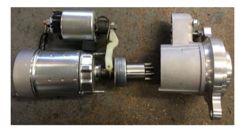
There is a thin slip ring. This must be between the c-clips and the planetary gear box, NOT between the drive and the c-clips.
