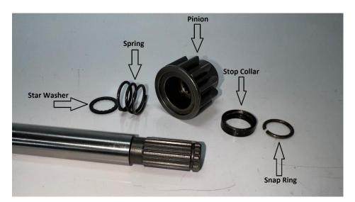
LMPK\*\*\*\* denotes the part is a pinion kit, the first two numbers denote the number of teeth on the pinion and the final two numbers denote the diameter of the gear. The letter suffix after is for short (S) 6.5mm nose, medium (M) 2mm nose & long (L) 0mm nose.
